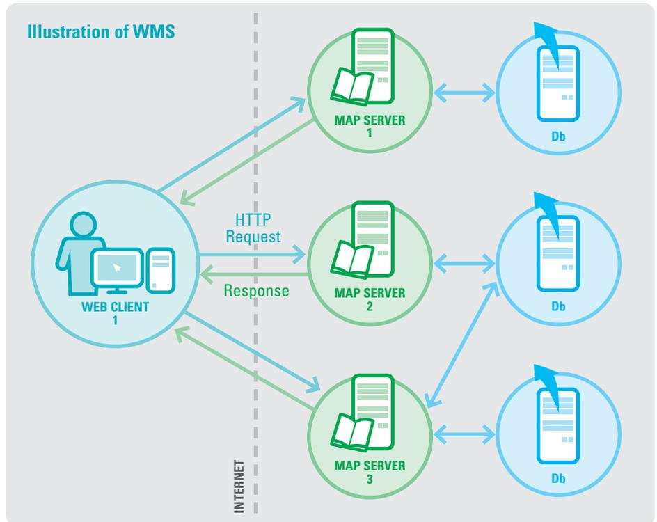
An optional third operation (GetFeatureInfo) provides access to information about displayed map features. With this option the features 'behind' the map can be queried, and their properties can be returned to a requesting client i.e. the user selects a point, line or polygon feature on the map to display further information about that feature.
