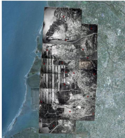
**Figure 12. Result of 2D projective transformation**
