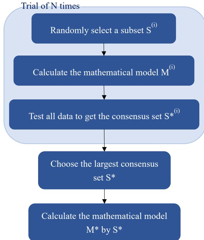
Figure 8. The flowchart of improved RANSAC
